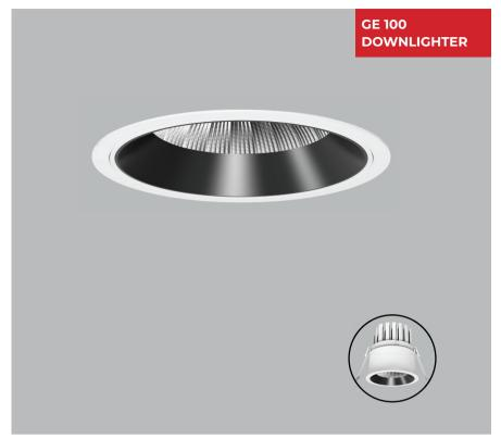
**GE 100** Recessed COB Spot light Downlighter is Fixed led Downlight made up of die cast aluminium housing, Finned heat sink to dissipate heat, increase performance and with premium powder coated finish.
